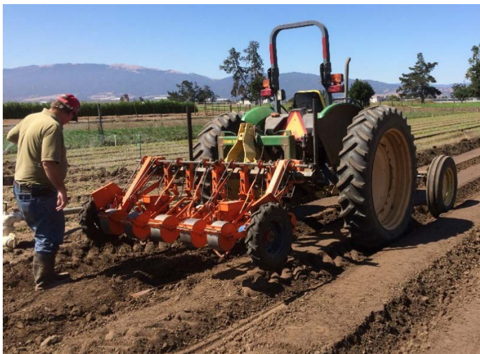
Figure 2.18. Stanhay planter used for direct seeding lettuce
