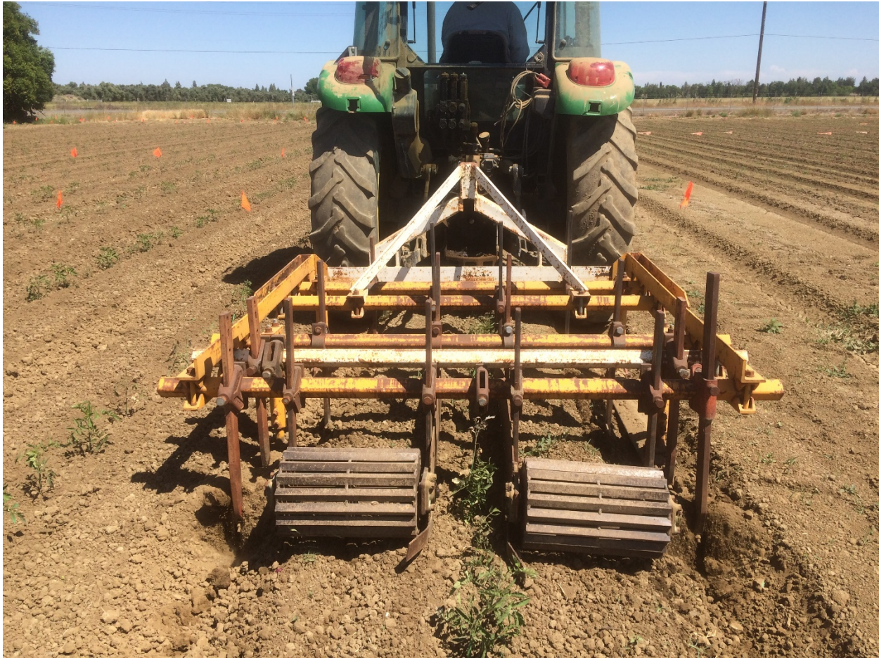
Figure 2.17. Standard cultivator setup for tomatoes
