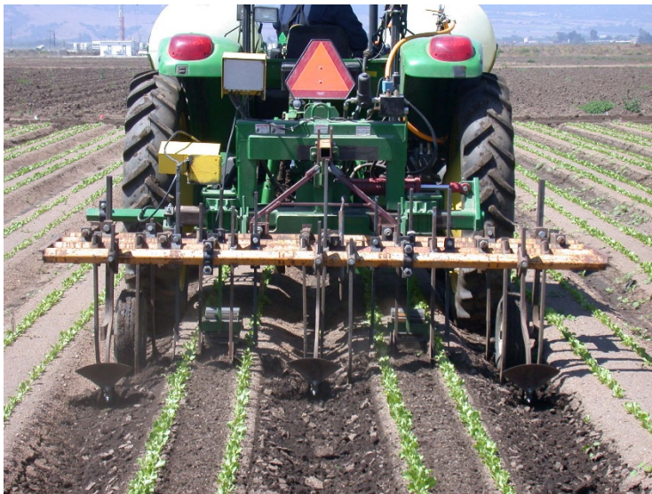
Figure 2.22. Standard cultivator setup for lettuce
