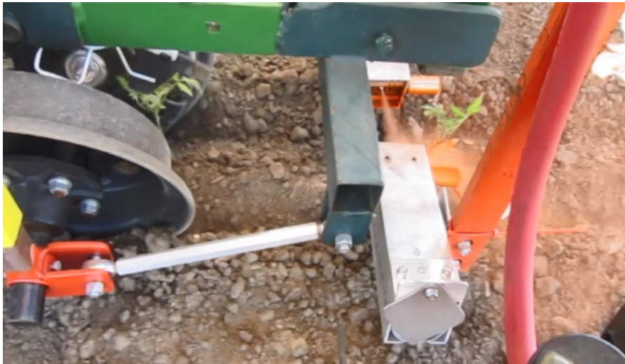
Figure 2.12. Topical marker spray applicator mounted on back of tomato transplanter.
