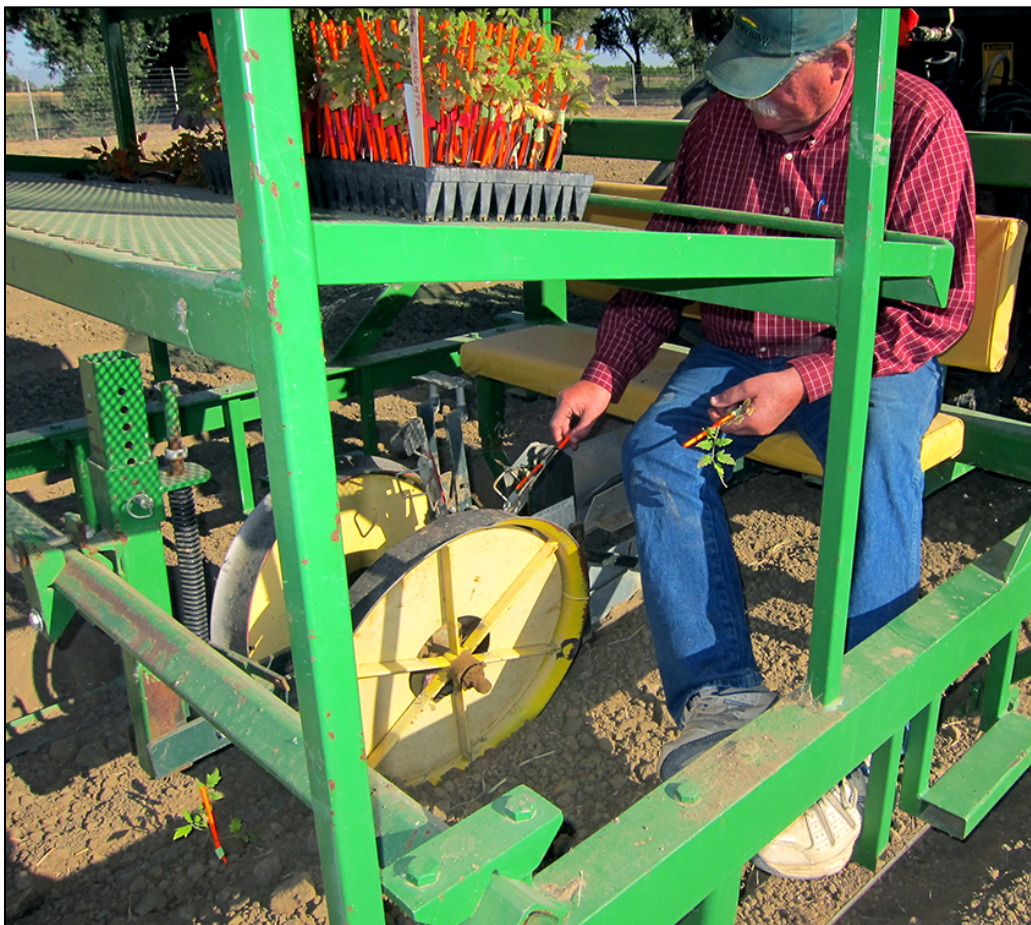
Figure 2.14. New Holland Transplanter with butterfly transfer fingers used for transplanting tomatoes. Shown here transplanting tomatoes with physical markers.
