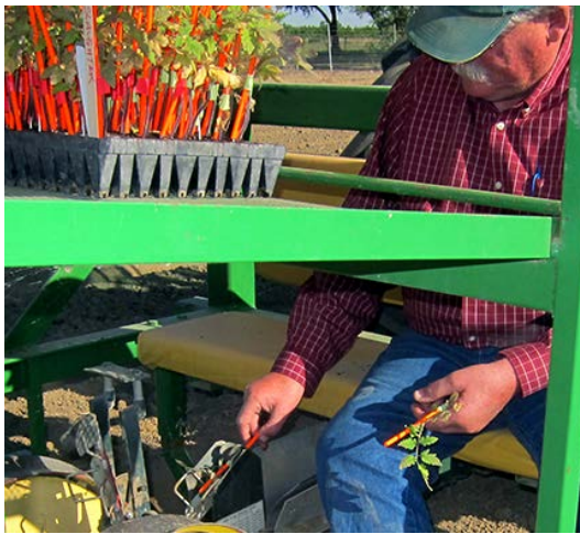
Figure 2.2a. Plant label being placed in tomato transplanter fingers
