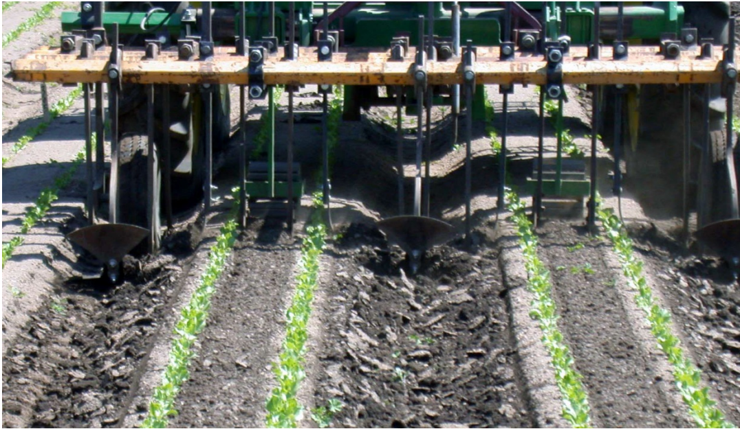
Figure 2.23. Detail of standard cultivator setup for lettuce
