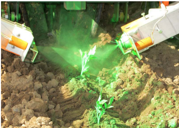
Figure 2.13. Topical marker being sprayed on tomato transplant by applicator mounted the transplanter.
